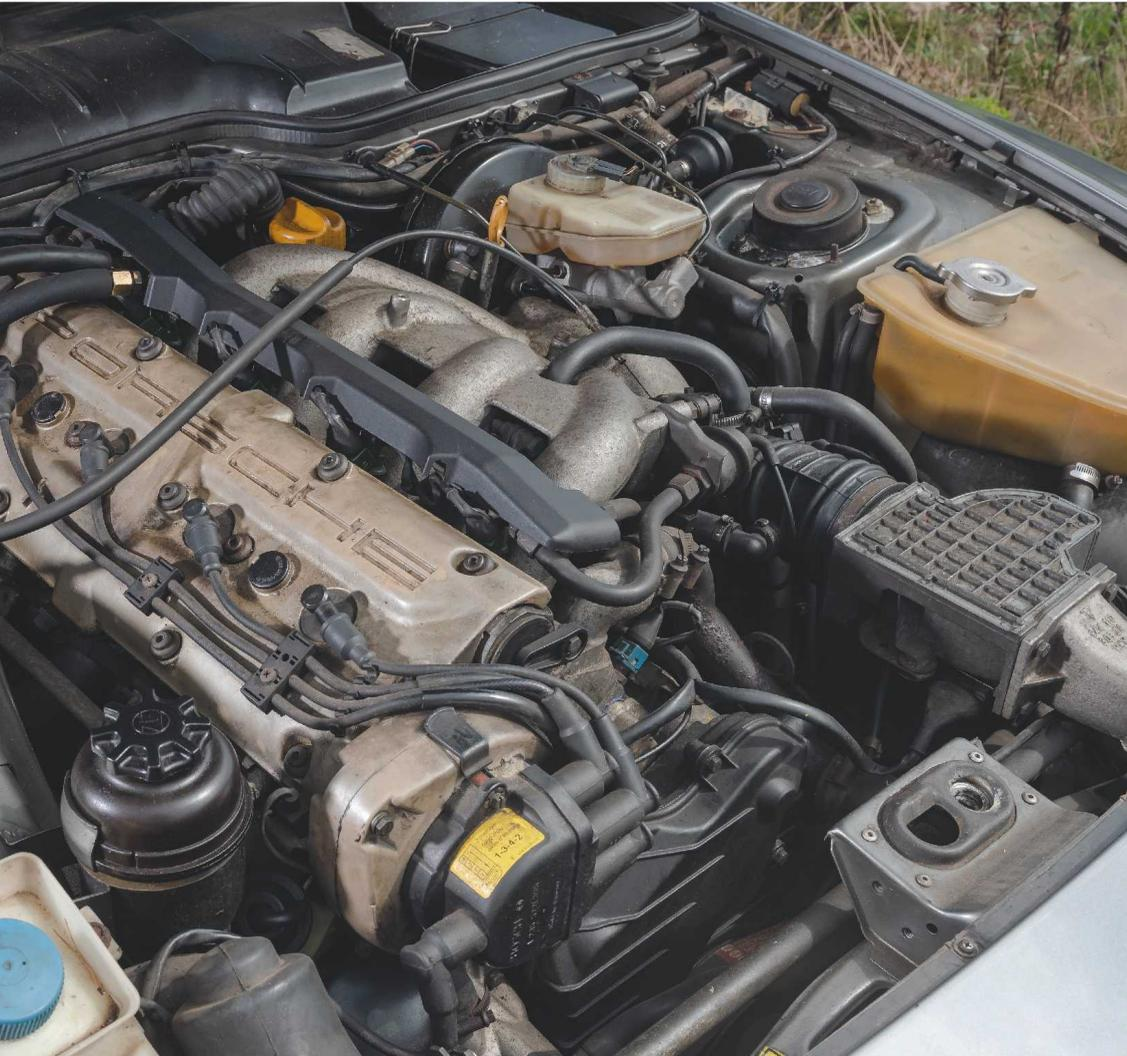
**Left** 944 engines came in a range of displacements, from 2.5-litres up to the pre-968 three-litre unit seen here
